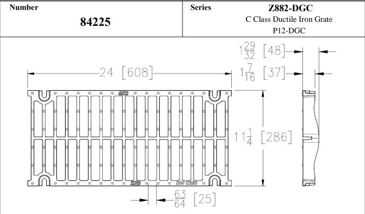
The Zurn P12-DGC Slotted Grate, Ductile Iron, is 11-1/4 inches wide by 24 inches long, weighing 14.7 lbs per linear foot. The grate has an open area of 86.7 square inches per linear foot, DIN Rating of C, ANSI Rating of Heavy-Duty, H-20 Load Rated. Supplied by Trench Drain Supply.
