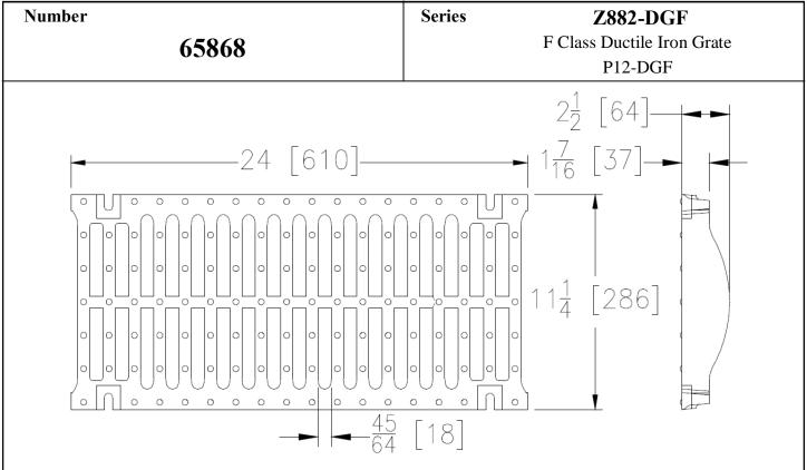
The Zurn P12-DGF Slotted Grate, Ductile Iron, is 11-1/4 inches wide by 24 inches long, weighing 26 lbs per linear foot. The grate has an open area of 54 square inches per linear foot, DIN Rating of F, ANSI Rating of Special-Duty, H-20 Load Rated, FAA Load Rated. Supplied by Trench Drain Supply.
