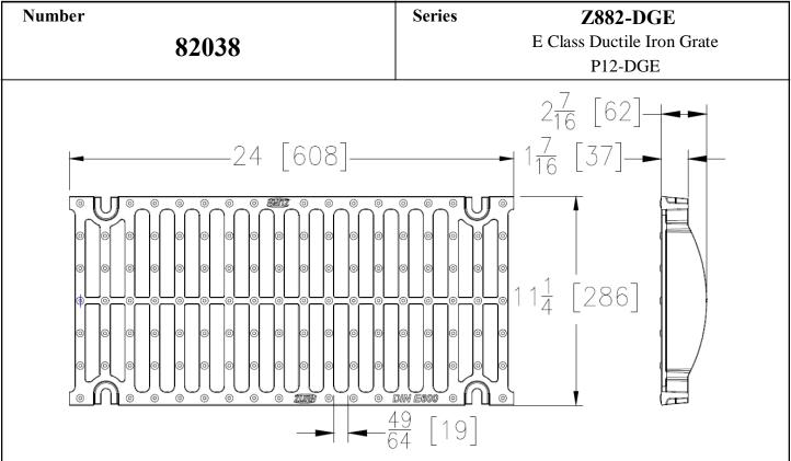
The Zurn P12-DGE Slotted Grate, Ductile Iron, is 11-1/4 inches wide by 24 inches long, weighing 19.8 lbs per linear foot. The grate has an open area of 60.3 square inches per linear foot, DIN Rating of E, ANSI Rating of Special-Duty, H-20 Load Rated, FAA Load Rated. Supplied by Trench Drain Supply.
