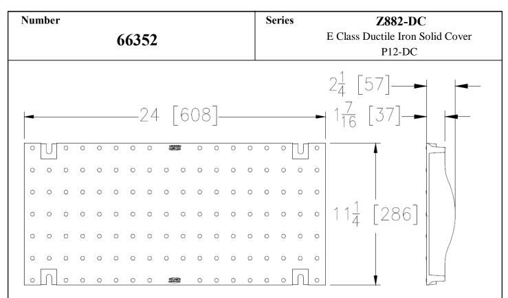
The Zurn P12-DC Solid Cover, Ductile Iron, is 11-1/4 inches wide by 24 inches long, weighing 27.9 lbs per linear foot. The solid cover has a DIN Rating of E, ANSI Rating of Special-Duty, ADA Compliant, H-20 Load Rated and FAA Load Rated. Supplied by Trench Drain Supply.
